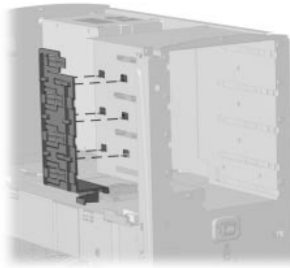
Removing the Drive Release Latch from the Drive Cage
