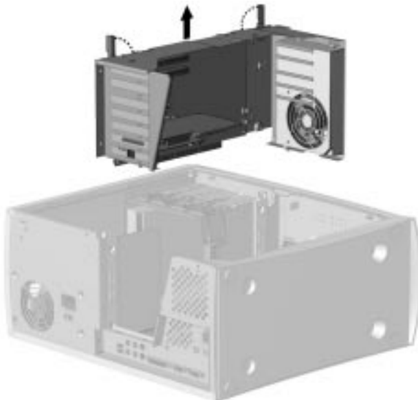
Removing the Expansion Board Cage
