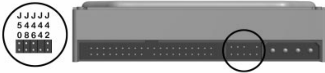
Maxtor Ultra ATA Hard Drive Jumper Settings
