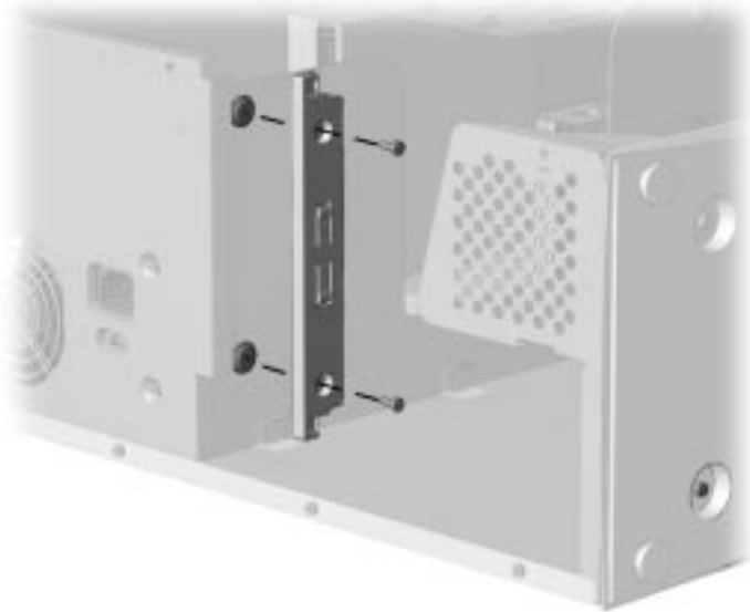
Removing the Expansion Board Cage Chassis-Mounted Guide Bracket
