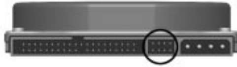
Seagate, Fujitsu, and Western Digital Ultra ATA Hard Drive Jumper Settings
